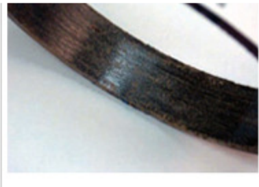
Fig. 9 Close up view of bushing center of contact surface
